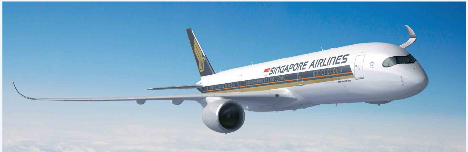
New generation aircraft such as the Airbus A350 (pictured) are around 25% more fuel efficient than older generation aircraft that they replace.
